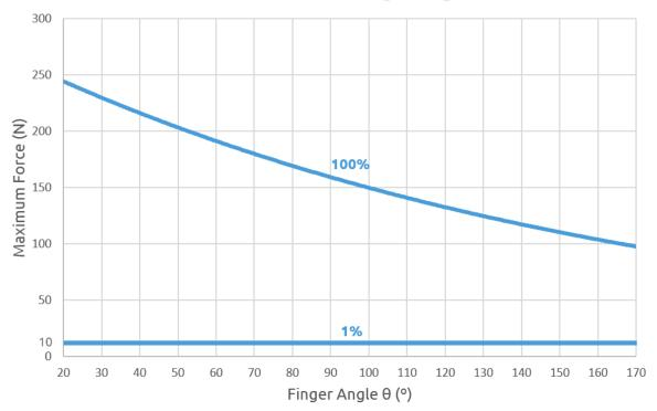
Graph plotted using measurements with 1 A current, silicone fingertips and a metal workpiece.
