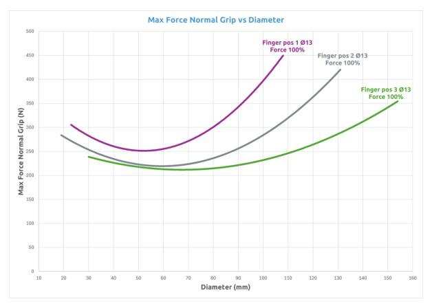
The graph below shows what force can be achieved for a specific diameter depending on the finger position when using the Flexible grip function. 300 N is the max posible value and under no circunstances this value is exceeded. The graph is plotted using measurements with the standard fingers in all 3 positions, steel fingertips Ø13 mm and a metal workpiece.
