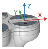
The maximum allowed torque applied to the gripper finger end around X and Y is 8 Nm.
