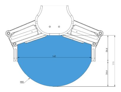
Gripping on long objects can unintentionally activate the Safety switches. The maximum workpiece height (calculated from the end of the fingertips) is dependent on the gripping width (w). For various width values the height (h) limit is given below:
